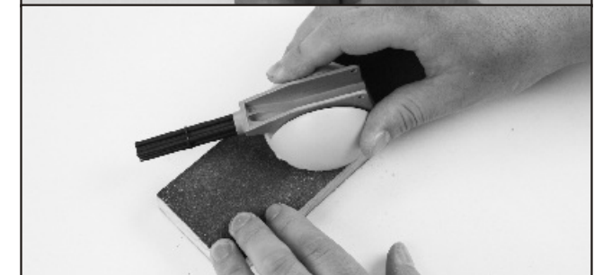
5. Trial fit the Turret Base in the Gun Turret, slight sand the contact area to improve the adhesion. Then epoxy the base in the turret. You may need to sand the base to make sure it is level with the rim.
