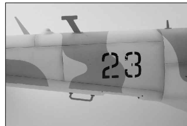
15. Install the scale fittings on tail fuselage includes Aerial Lean-in, VHF Aerial, UHF Aerial Mast and Aerial Cable. Drill 2mm holes at the proper position then secure the fittings firmly with collars as shown. Then glue them in place.
