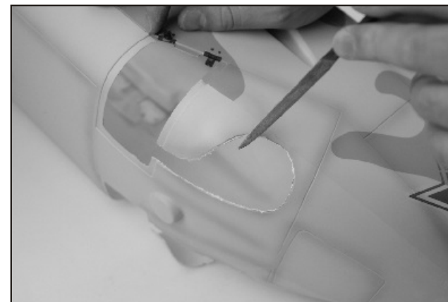
26. Do the "Cut-out" along the molded line for retract gear on the bottom fuselage. A half-round file will help on doing this. Do the same way on the other retract gear area.
