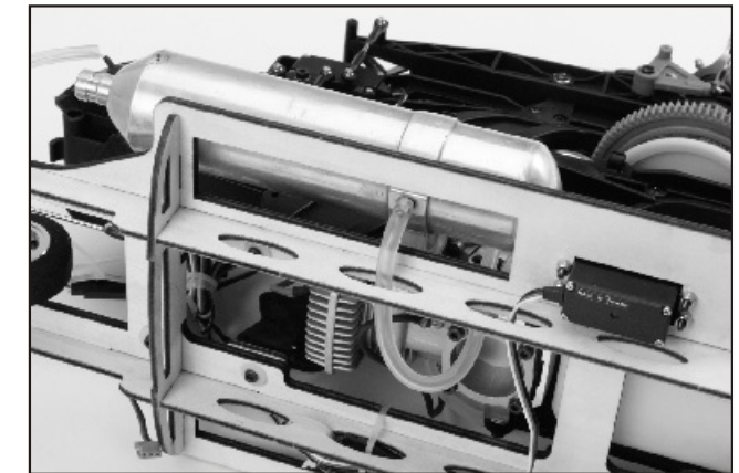
75. Suggested to use the muffler (PV0109) which comes with Titan, if user use other brand muffler then the muffler may contact the fuselage or wood mount, even contact the servos. Remove the muffler and install the muffler reversely. Well connect the pressure tube to the fuel tank. (Titan SE includes a black muffler which will contract the servo and need to replace a silver one)
