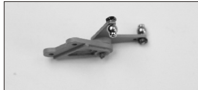
92. Install the ball bearing and collar in the Bell Crank next secure the bell crank on the Bell Crank Mount with two M3 washers and 3x10 self tapping screw. Make sure bell crank moves freely. Next install the two balls on the bell crank with 2x8mm screw and M2 nuts. Two balls are on the different sides as shown.
