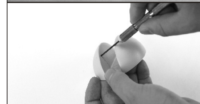
3. Drill two pilot holes on the Turret as indicated position then enlarge up to 3mm (1/8") in diameter.
