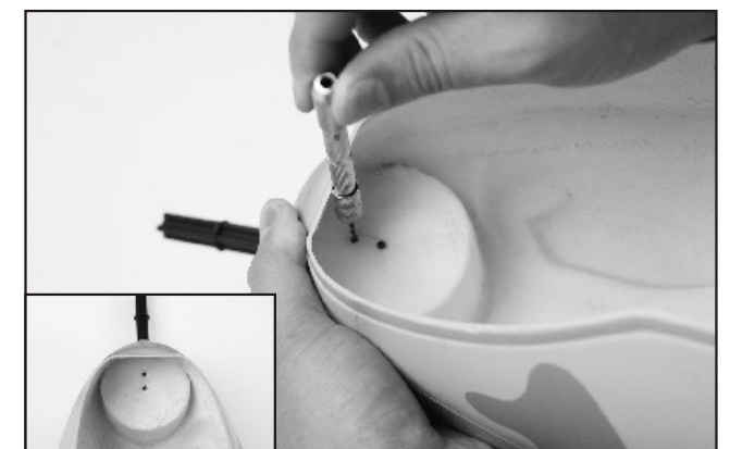
6. Secure the Machine Gun assembly onto the nose bottom of the front fuselage with two 2x8mm wood screws.
