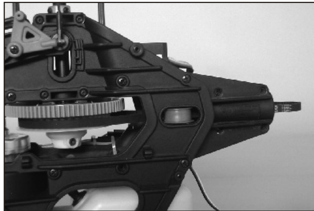
67. Remove the tail boom and old belt. Install the new short belt as shown.
