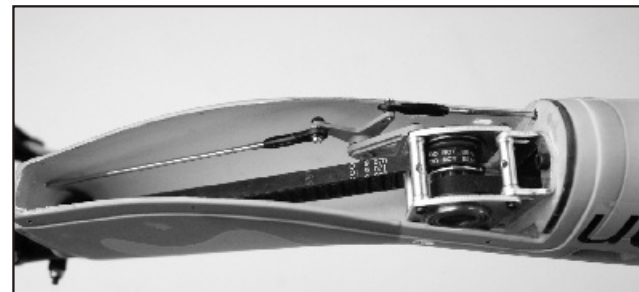
93. Remove the two screws on post C then install the bell crank on the bearing support as shown. Now you can secure the bearing support firmly in place. Do not forget to apply Loctite. Next assemble the pushrods and snap onto the balls on bell crank.
