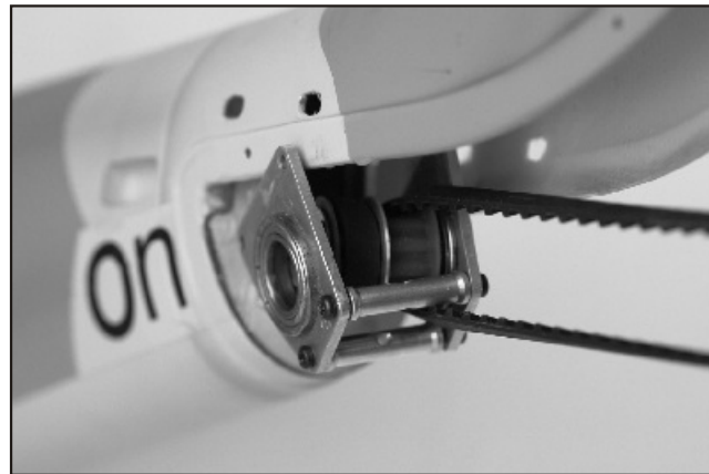
81. Move the mechanism all the way in then try to get the long belt. Refer to step 79 and assemble the pulley with the belt in the bearing support. Before securing the bearing support in place you will need trim four holes on the tail at the molded line. These holes are for screw drivers to go through to secure the screws.
