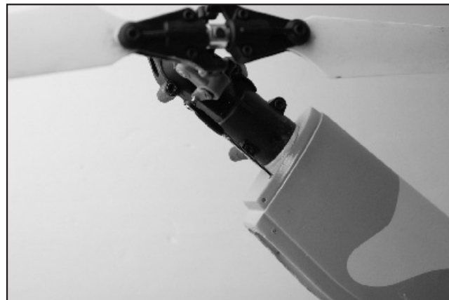
95. Snap on the pushrod ball end on the tail blade pitch control level. Adjust tail pitch as you test flight the Titan.
