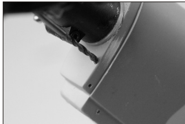
91. Drill the pushrod exit hole at the tail end.
