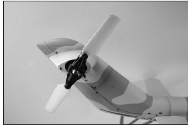
107. Finally secure the fin tip in place with eight pieces 2x5mm setscrews.
