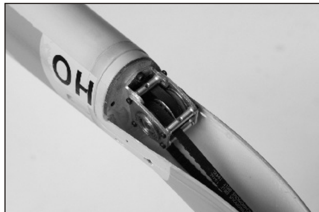
82. Temporarily secure bearing support all the way to the front in place. This step is very important before you glue the integrated wood mount in place.
