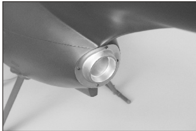
28. Secure the exhaust vent in the place with four 2x5mm wood screws as shown.
