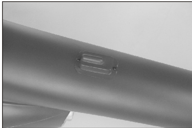
25. Locate the vacuum formed decoration and place it at the center line of the tail section. Drill two 1/16" (1.5mm) mounting holes and secure it with two 2x5mm Wood Screws.
