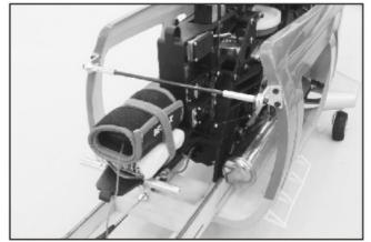
33. Assemble the carbon rod with two rod ends. Next install the other two body retainers and carbon rod with two 3x8mm, four 3x10mm socket screws, M3 washers and locknuts.
