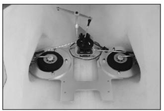
18. Install the retract you just removed from the main plate as shown.
