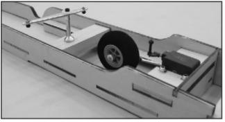
12. Same way to install the front horn in place with 3x6 and 20mm socket screw, M3 washer and POM washer, two 8mm standoff- balls. Install the nose gear in place with 3x10mm sink head screws, M3 washer and locknuts. Secure the 18mm standoff-balls on the nose gear pushrod with M2 nut.
