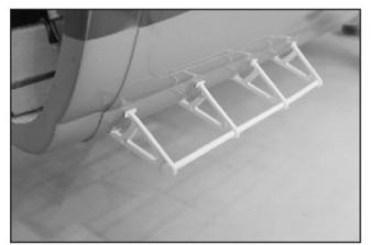
28. Locate foot step accessories then use care to install the foot step support on the fuselage, make sure they are level with each other. Press the retaining collar firmly then apply CA at the last.
