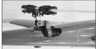
39. Install the tail in place and trim the contact areas with tail transmission.
