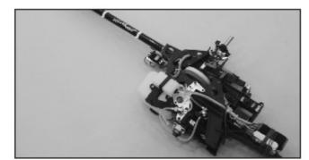
1. Get your Raptor 90 well tuned before you install the body. Remove the tail transmission, landing skid and rotor head.
