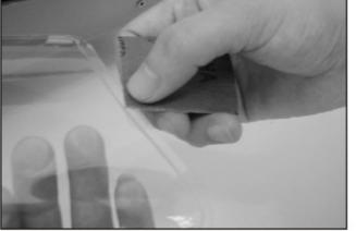
48. Trim all windows and both sand the glue area on windowsand fuselage. Epoxy the windows in place properly. You mayskip installing the middle window for engine adjustment and any maintenance of helicopter.
