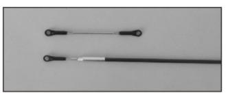
13. Assemble the pushrods; one is about 95mm between two center points of ball end, the other is about 465mm of two ball end center.
