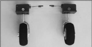
3. Secure the main retract wire with the setscrew which is already in the retract shaft. Adjust the wire at 50mm (1-31/32") in length then insert POM washer, wheel then secure the collar with setscrew.
