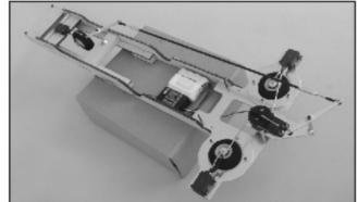
14. Temporally install the retract assembly on the wood mount then install the pushrods to link the front and rear horn as well as the nose gear pushrod. Test the retract gear and adjust the pushrods until it works perfectly.
