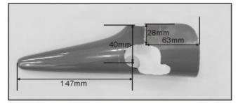
38. Cut tail end into two pieces as shown. Use the template in page 15, cut the template off and apply on tail end then trim off the area.
