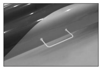
16. Install the handle rail at the tail, it is about 27cm from the end. Drill 2mm holes and press plastic collar to secure it in place. Apply tiny CA at the contact area of handle rail and fuselage.
