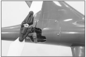
40. Secure the tail end with 2x5mm wood screws.
