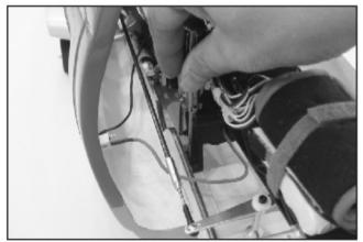
30. Before you install the helicopter into fuselage, get an extension wire for retract servo. Carefully install the helicopter in the fuselage, pull the tail boom and position the helicopter in place properly. Secure the helicopter with 3x35mm socket screw, POM washer and M3 Locknut.
