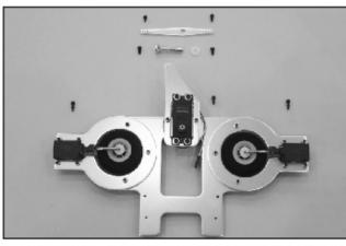
7. Install the retract gear on main plate as well as the retract servo, note the servo orientation. Locate the two 12mm standoff-balls for retract pushrod; 8 and 10mm standoff-balls, standoff, 3x6mm socket screws and POM washer for rear horn. Note the rear horn is longer than front horn.
