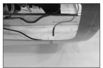
31. Install the ignition extension outlet on fuselage.
