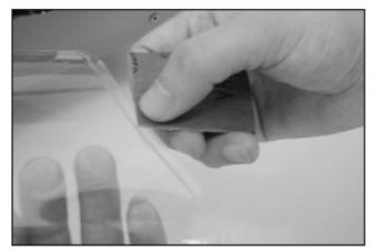
41. Trim all windshield and windows. Both sand the glue area to enhance the adhesion. You may skip installing the middle windows for easy access and tuning the helicopter. This also help the cooling.
