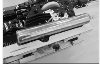
21. Install the muffler and check if muffler contacts the wood mount. You may need to trim the wood mount. (photos shown is OS91 with Zimmermn muffler) The kits comes with muffler extension that you may use. Check if the throttle lever contacts the muffler if you use the extension. Trim the contact area if necessary.
