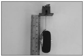
4. Same way to assemble the nose gear and adjust the wire at 65mm( 2-1/2 ") in length.
