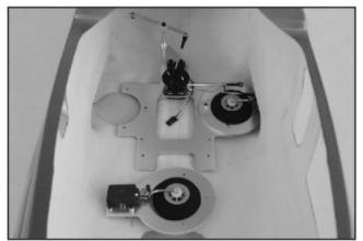
17. Remove the retract assembly from wood mount. Next remove one side of retract from main plate so it could be placed in the retract area of the fuselage.
