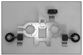
6.Secure the retract mount and the servo tray on the main plate. Next locate retract gear, 3x10mm sink head screw, M3 locknut, retract servo, 3x12mm socket screw, M3 locknut and washer as shown.
