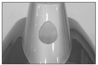
42. Epoxy the small screen inside the front fuselage as shown.
