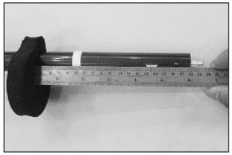
29. Locate the tail boom foam retainer, measure at 18cm(7") from the boom end. Secure foam retainer in place with CA.
