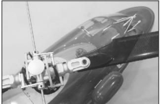
50. Cut the front fuselage then join the front fuselage to the rear fuselage with 16 pieces of 2x5mm wood screws.
