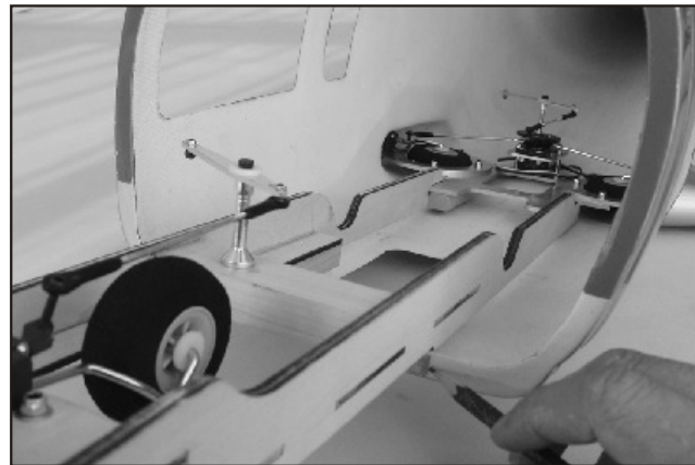
19. Place the wood mount and join the main plate, next center the wood mount then make marks on fuselage.
