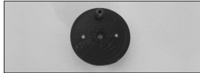
10. Get a disc horn then drill two 2mm hole ( 9.5mm to the center) as photo shown. Drill another 1.5mm hole (16mm to the center) then secure the 10mm standoff-ball with M2 nut.
