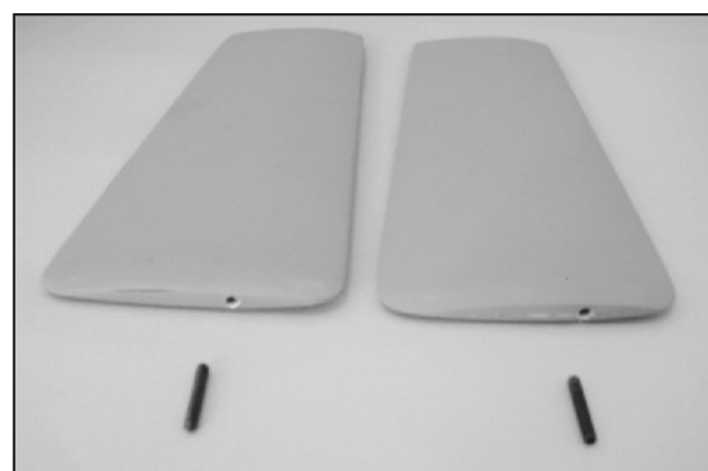
35. Locate 3x25mm setscrews then install on horizontal tail. Apply epoxy inside the hole and thread the setscrew in the tail and leave about 10mm in length outside the tail.
