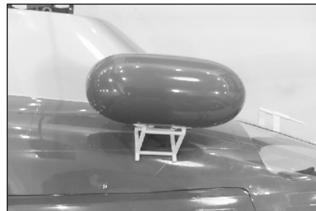
47. Next install the hoist assembly on the fuselage as photo shown.
