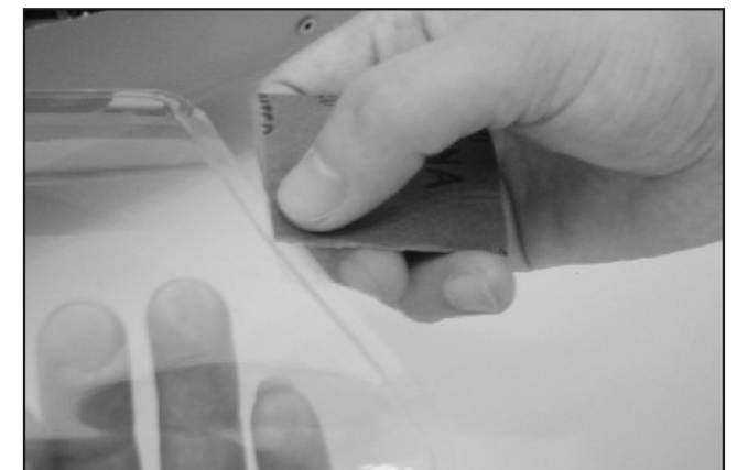
41. Trim all windshield and windows. Both sand the glue area to enhance the adhesion. You may skip installing the middle windows for easy access and tuning the helicopter. This also help the cooling.
