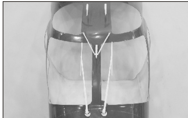
44. Install the wipers, upper wire strike and antennas in front of the windshield as photo shown.
