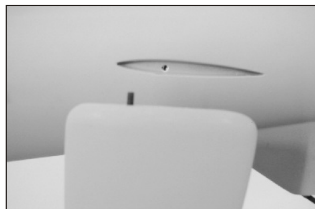
36. Drill a hole to accommodate the setscrew on tail. Trial fit the tail in place, lightly sand the glue area then epoxy the tails in place firmly.
