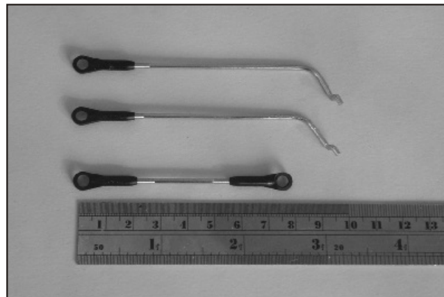
9. Locate the Z-bend pushrod and 45mm threaded rod then thread the ball ends. Measure at two ball ends at about 75mm.
