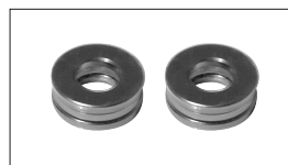
PV0365 THRUST BEARING, d6xD12xW4.5 止推軸承組, d6xD12xW4.5
