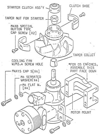
Remove the prop drive hub from the engine crankshaft and install the split tapered collet in its place.
