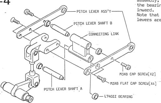
On the pitch lever A assembly, the flange of the bearings are faced inward.
