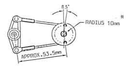
When installing the rods into the servo horns, first determine the best side of horn to use as the height of the servos differ by manufacturer.
