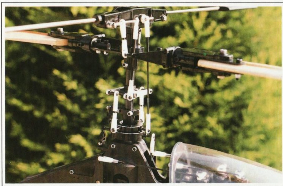
Close up showing the rotor head and collective/swashplate assembly. Note the aerobatic mixing levers.
