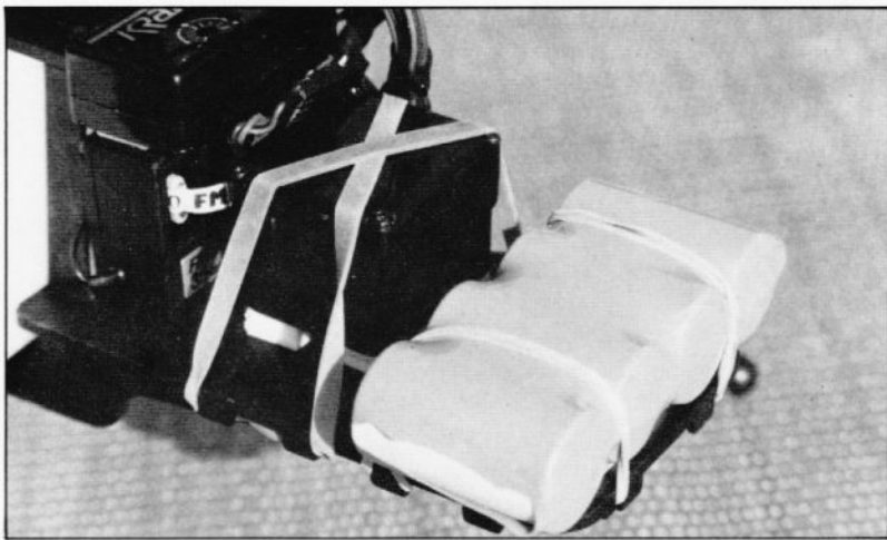
Showing placement of receiver, battery and in the reviewers case gyro.
