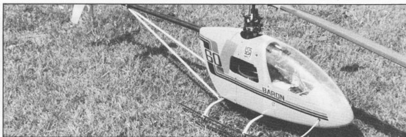
The Baron 60 with its unusual egg-shaped fuselage.
