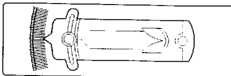
Pitch gauge (This is used to measure the collective pitch angle of the main rotor blade.) (0002-030-8)
