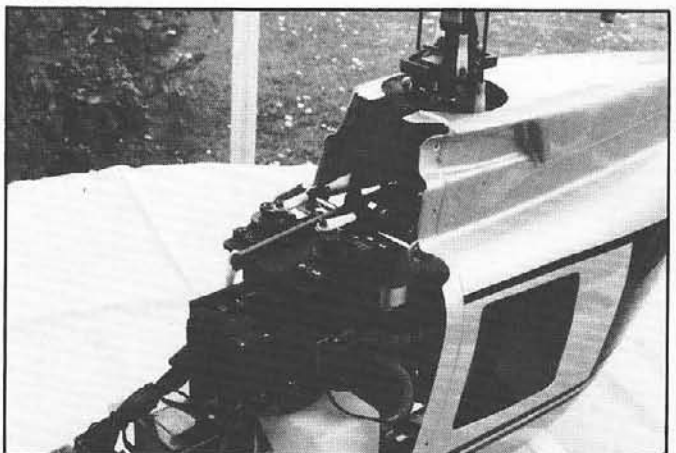
See how the fuselage is screwed to the original canopy mounts.
