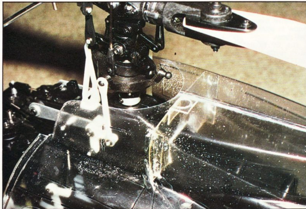
Underside Access: This view shows the cut-out to provide outlet area for the cooling air and access to rear cone start belt starting using longer belt provided in kit should not be a problem, although window/ body cut-outs could become damaged as the belt 'flaps' in use.
