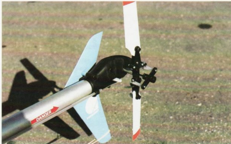
Standard production Hirobo tail rotor parts. Moulded tail tube and houses bearing supported output shaft and cog pulley. Large diameter tail tube needed to enclose cog belt.
