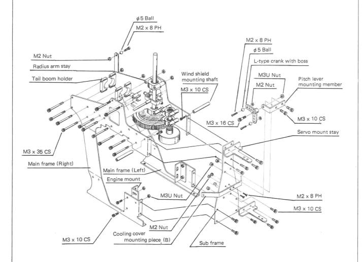
NB: Tighten the whole section more after the engagement of the bevelled spur gears is sufficiently checked.
