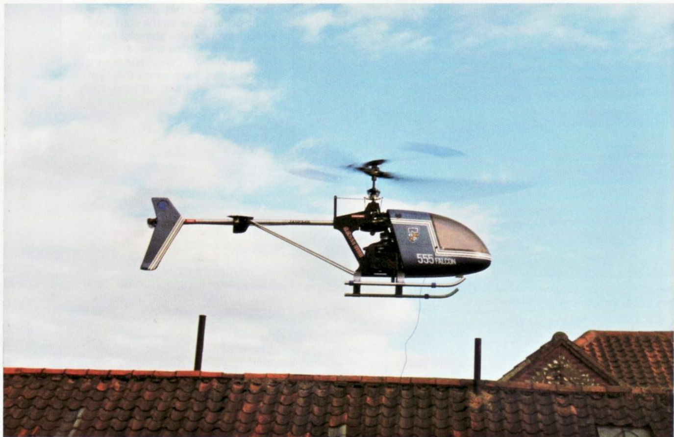
The model in a steady hover after final trimming. The tail is reasonably powerful and with the help of a gyro anyone could learn to fly with it, as they could the same with GMP's Cobra. Photos by Diana Cameron-Tough
