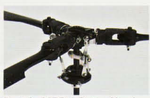
Shuttle MRB-III Rotor Head Conversion Set 0402-135 This conversion set includes MRB rotor head, main blade, swash plate, etc. which are used for remodelling SHUTTLE to three-rotor type.
