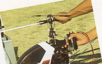
Shuttle Z-Series Conversion Set 0402-218 Parts set for converting standard/ XX type Shuttle into Z Type. Set including: FZ rotor head assy 0402-214, CG balanced stabilizer blade 0402-208, Main Mast 0402-207, Inside tail pitch plate 0402-205, Inside tail housing 0402-216, Inside tail drive shaft 0402-204, Inside tail pitch lever 0402-206
