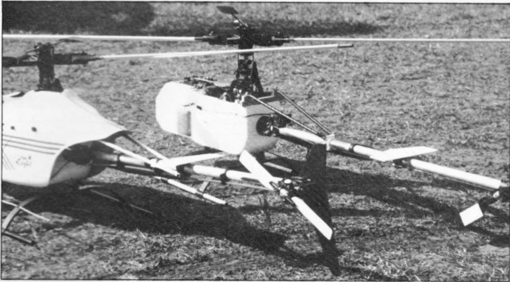
Starlight on right, Trainer on left. Notice different tail boom layouts.
