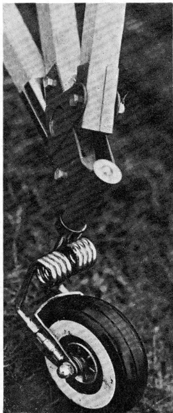
A modification to the training undercarriage is to fit castoring wheels. These are essential as, at first, one is never sure in which direction the model will skate off, or land, come to that, and fixed wheels would cause the 'copter to tip over more readily, which will break a rotor blade or, at the very least, bend the blade mounting plates and the stabilizer blade rod, necessitating a return to the workshop for repairs and re-alignment. Standard steerable nosegear is easily modified, as shown right.
