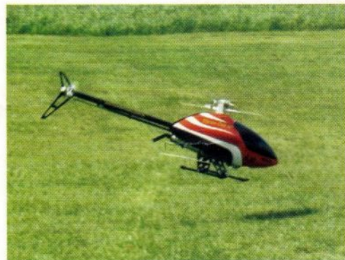
The light weight produces superb auto performance with a slow descent giving time to think!
