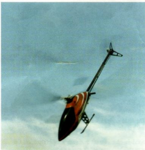
The NT is at its best in forward/backwards manoeuvres, the large side area slightly limits sideways loops.
