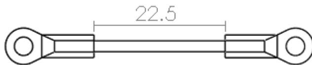
No.4 T-arm servo (L) Control (L=40 for 120ccpm, L=25 for 140ccpm)
