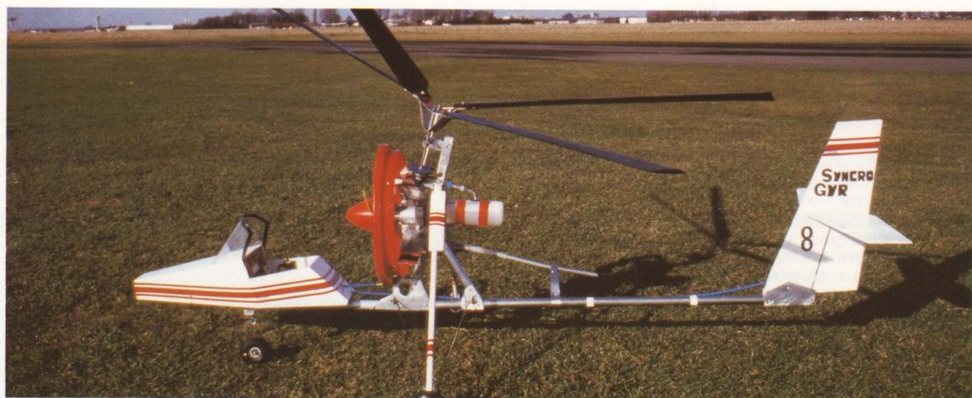
One of Georges Chaulet's most interesting Gyroplanes, with simplicity the key word – it was called 'Synchrogyro 8', and was the 68th one he built, with an OS .90 engine it weighed in at 7lb.
