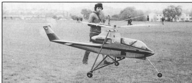
A young Vago Nordigian with one of the original Schlüter Tow Cobras with the tricycle undercarriage – ideal for training. He doesn't care to say how long ago the photograph was taken!
