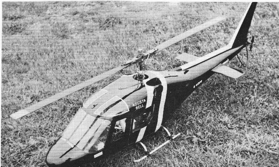
Sean Wiles' Augusta 109, featuring Kalt GS22 mechanics and a flybarless rotor head, shown above in close up.
