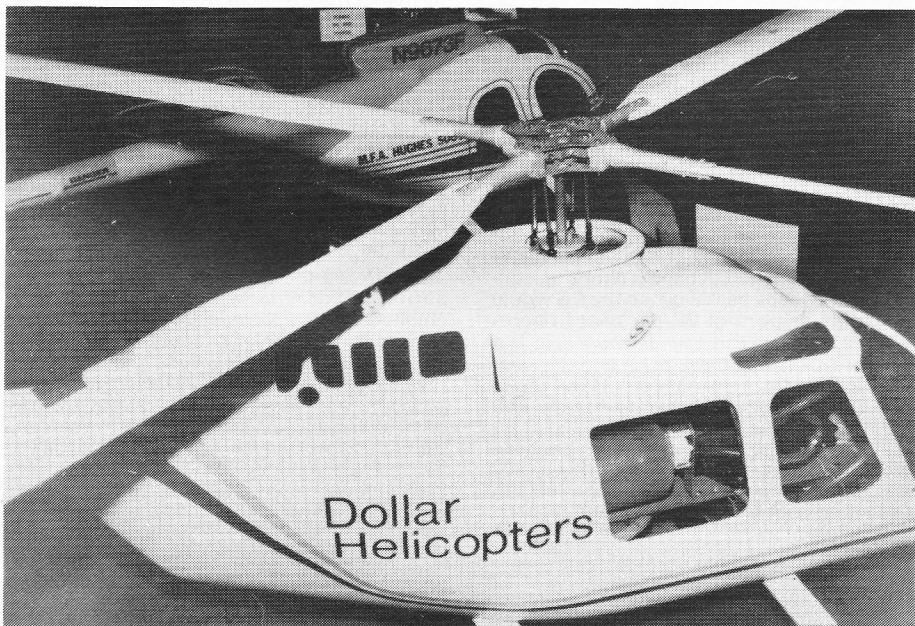
Above: unusual 'Jet Ranger' built by P. G. Noel of Hertford and exhibited at the ME Exhibition features a Schlüter type four-bladed head.
