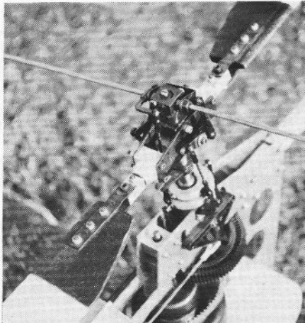
Below: glass fibre cloth and metal strip reinforcement to the blade roots are visible on this machine.
