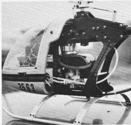
Above the Baron 20 tested by your columnist, which has proved itself capable of lifting an Action Man jeep, as shown right. Below: the mechanics of the Baron 20 and left: the modified head which now employs cut down paddles and wheel collets to compensate for the lost weight. It should be noted that fly-bar modifications are quite fundamental and should be treated with the respect that serious changes deserve.
