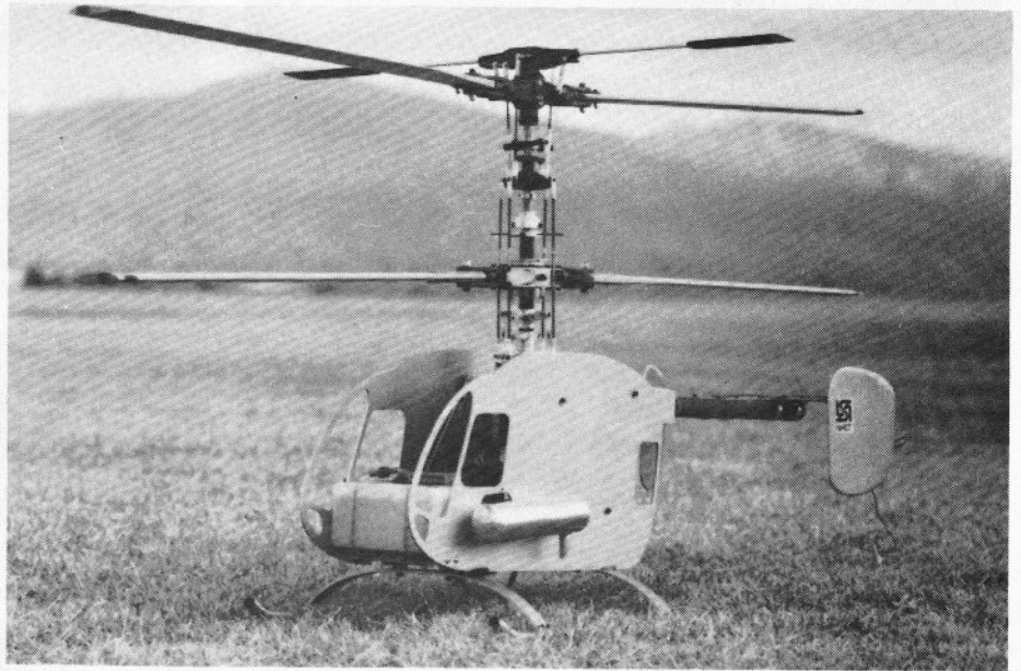
Above: interesting prototype in Japan. Shape of things to come? Uses all Kalt mechanics. Contra rotating rotors eliminate the necessity for torque compensating tail rotor.
