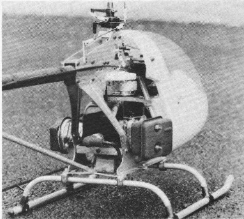
Left: Kalt Baron with 22cc petrol motor. Looks the part and apparently sounds like a Bell 47g flying around. Right: Prototype of another new helicopter, the Morley Mk 3. Intended to be an 'easy build' kit. Should be available during the summer.
