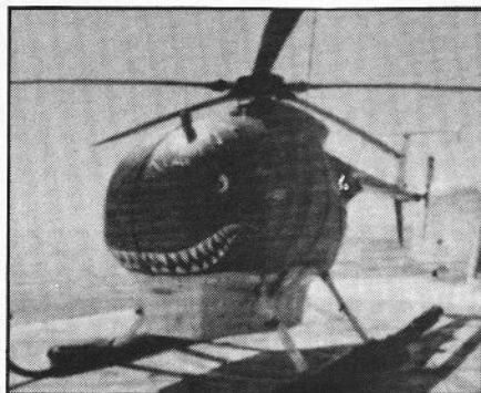
Left: Mick Harris made this three bladed rotor using Kalt blade mounts.
