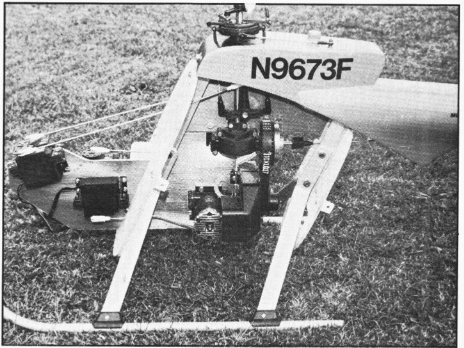
Above: the Model Flight Accessories Hughes 500D has a body shell that comes away in two halves to enable easy building and maintenance of the mechanics, but the tail rotor drive down the boom needs care. There is a shallow "S" bend as the drive goes up and to the side which can control the "whirling" and "wind-up" of the wire in this type of drive.
