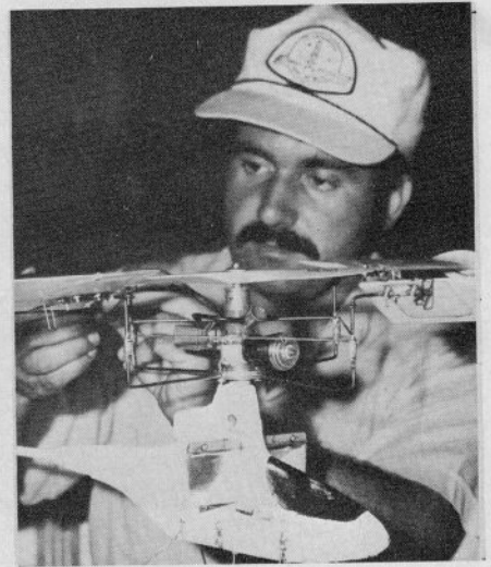
Navy photo of another FF chopper flier, Tony Naccarato, Jr. It is 049-powered and a fairly simple configuration. Climbs very fast.
