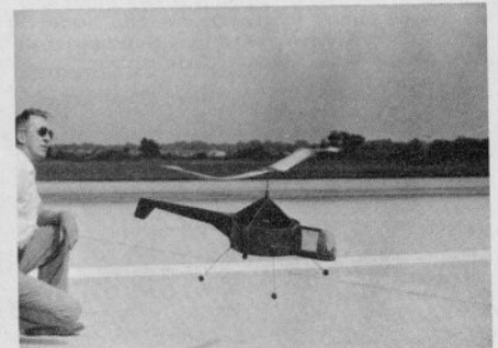
Glen Lee's large 15-powered FF model has low disc loading and so its sink rate in autorotation is very slow. Engine is on the main shaft for torque reaction drive but located below and inside the fuselage.
