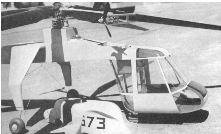
Below: Rotor head fairing, hatch shown removed. Design is of interest to all builders in approach to variety of unusual helicopter problems.
