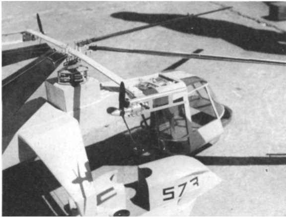
Above: Three bladed props for cabin clearance, as two .049 Cox swing 99" rotor around. Designed in Denver, extreme altitude has been a big problem, slowed development. At right: Ken displays how blades are free to seek own level in flight. Cyclic and collective pitch, note four controlling flaps on blades.
