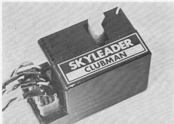
Clubman receiver features connector block for servos and power pack and employs two-deck p.c. layout. Crystal stands partially proud of case and should be carefully protected in any installation. Silicone compound support for components is a sensible feature.
