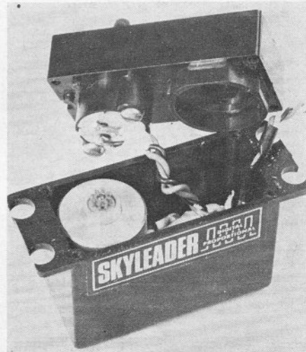
New Skyleader SRC servo can be used with either rotary or linear output. Units are supplied fitted out for rotary action, but case tops for linear drive are also provided for conversion.
