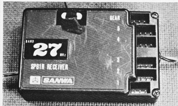
Heading shows the complete outfit, with carded crystals, harness, charger and servo trays. Close-up of receiver, above, shows crystal cover removed. Below is the "works" of the receiver, with p.c. board at right, about actual size.
