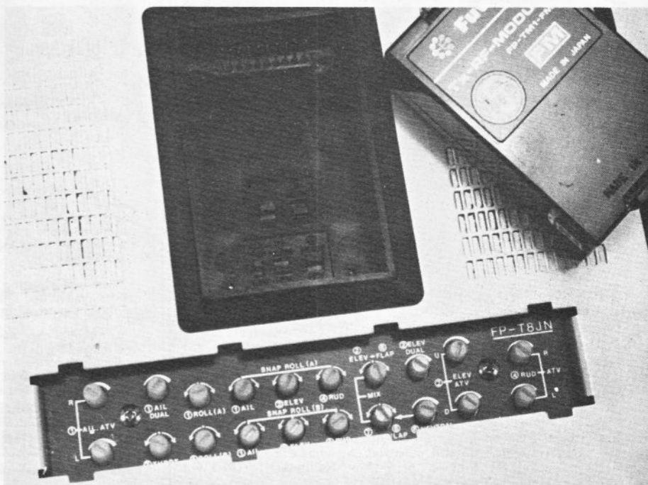
Above: only part of the array of switches and buttons are immediately visible, the remainder are tucked away beneath the Tx., R.F. module and a clip-in panel both shown removed below.
