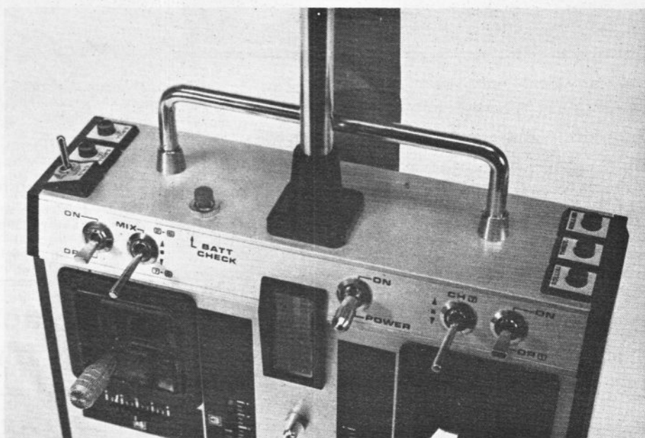
Above: only part of the array of switches and buttons are immediately visible, the remainder are tucked away beneath the Tx., R.F. module and a clip-in panel both shown removed below.
