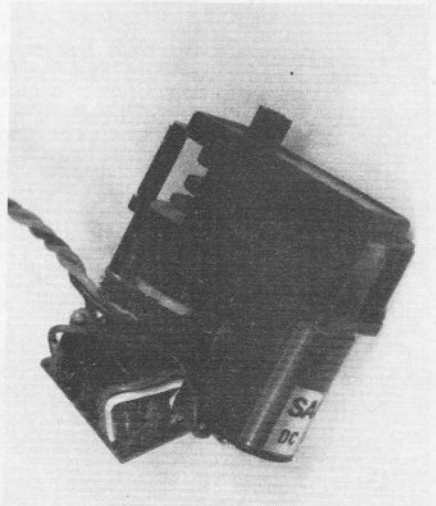
Above: Sanwa SM402 — note the ballrace mounted output shaft and the metal gears. The thin film IC is mounted edgewise on the amplifier PCB. Below: OS CS50 servo — the same mechanics are used for the World Engines D5. W.E. guarantee the geartrain for life!
