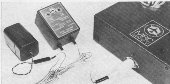
MRC 5 transmitter uses conventional two piece vinyl clad folded metal case. Position of retract switch depends on mode chosen—goes next to stick with throttle function. Internal layout is simple, sparse and tidy. Crystal immediately accessible after removal of case rear cover. Top right: servo trays, frequency pennant and several servo output arms are supplied with set as is charger and harness, 2nd right.
