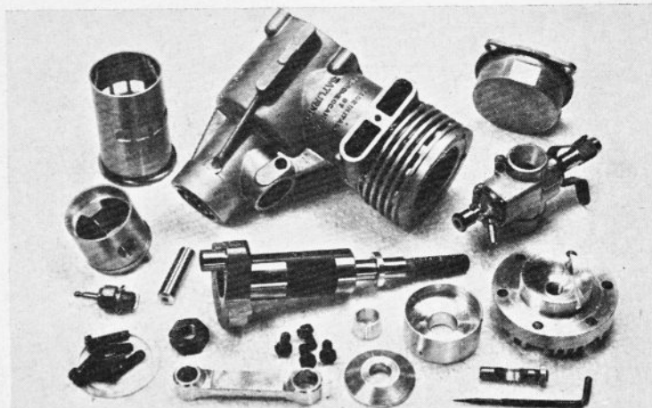
Parts of the Super-Tigre ST 51. Well built engine has large diameter crankshaft, chromed liner bell-shaped combustion chamber and easy-to-adjust carb with automatic mixture control.
