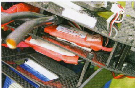
ESCs with a high refresh rate are essential although, surprisingly, they're often not the most expensive.
