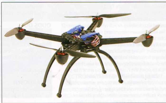
The iFly4 is an RTF machine requiring only your Rx and 3s Li-Po battery.
